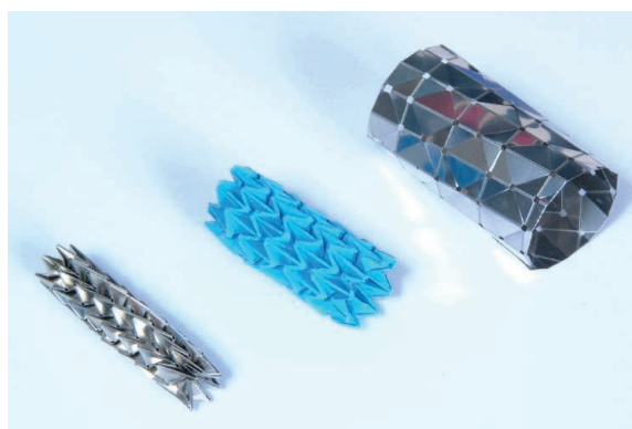
Insider. Creased stent is designed to snap open inside an artery.
